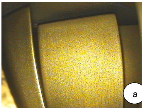
Figure 13. Suction side and trailing edge of compressor blades (7th stage) operated in the following conditions: a) "normal", b) heavy dust [4]
