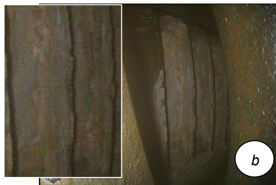
Figure 10. Gas turbine operated in the heavy dust conditions [4]. The accumulating, sealing up, and after some period of time tearing-off dust on the surfaces of the leading edges and troughs of aerofoils a) row of vanes, b) blades of the first stage
