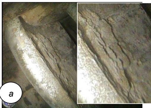
Figure 10. Gas turbine operated in the heavy dust conditions [4]. The accumulating, sealing up, and after some period of time tearing-off dust on the surfaces of the leading edges and troughs of aerofoils a) row of vanes, b) blades of the first stage
