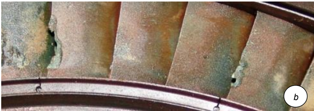
Figure 12. The removed first stage of the turbine stator (of gas generator) [5]. View in the direction of edges: a – leading, b – trailing
