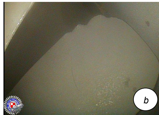
Figure 13. Suction side and trailing edge of compressor blades (7th stage) operated in the following conditions: a) "normal", b) heavy dust [4]
